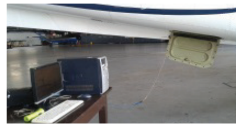
TRC-899 TCAS Computer configured for SMR-2311 (Proline-21) Beechcraft at No 8 Squadron Sri Lanka Air Force Base Rathmalana
