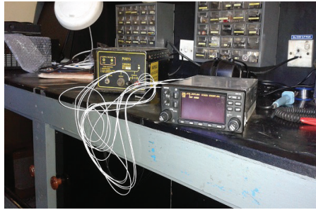
TRC-899 TCAS Computer configured for SMR-2311 (Proline-21) Beechcraft at No 8 Squadron Sri Lanka Air Force Base Rathmalana
