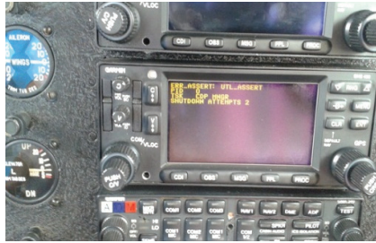
Local repair of GNS-430 System for SCL-3124 Y-12 IV aircraft at No 8 Squadron Sri Lanka Air Force Base Rathmalana
