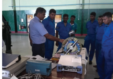
Major servicing of slip ring in the YLC-18M Radar Sri Lanka Air Force Academy China Bay by the SLAF Technical Team
