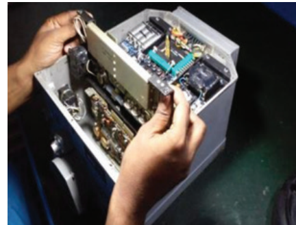
Local repair of Pilot Box for the Advanced Ground Control Station (AGCS) at Squadron Sri Lanka Air Force Vauniya
